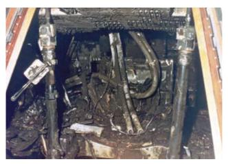
A close-up view of the interior of the Command Module shows the effects of the intense heat of the flash fire. Courtesy of NASA.
